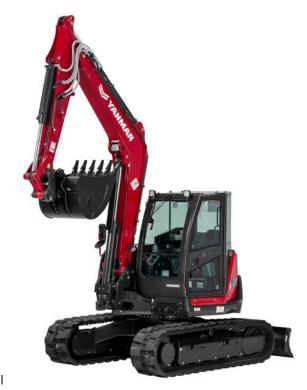
YANMAR's SV100-2A, our 10-ton class mini excavator, is powered by a 72 HP Tier 4 Final YANMAR engine. It is our largest, most powerful
