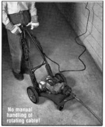
Cleans 3" to 10" diameter sewers, drains and industrial pipelines for distances over 200 feet!
