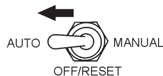
Figure 54. MPEC Control Switch (AUTO)
