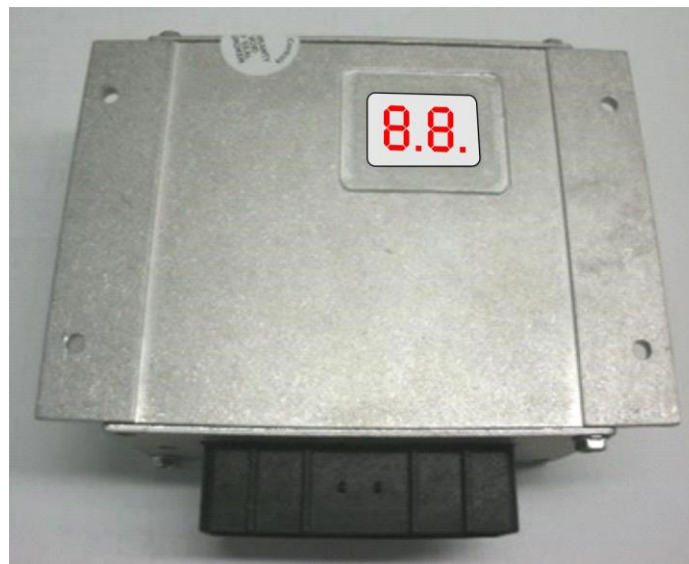
Figure 4 Electronic Control Unit (ECU)
