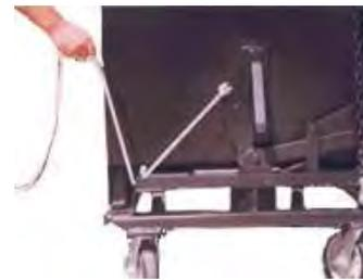
can be used to trip the hopper from the ground or from the operators seat.
